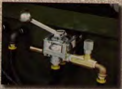
Direction and speed control valves
