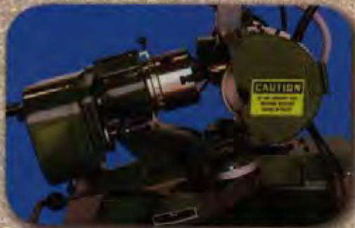
Benchtop version shown with workhead positioned for point splitting.
