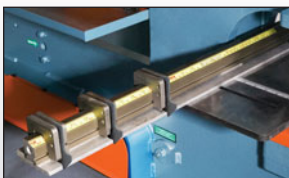
Multi-Loc Punch Gauging Extension: 36" & 85" (DD)
