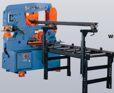
Multi-Loc Punch Gauging Extension: 36" & 85" (DD)
