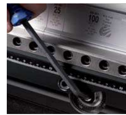
HF Manual in the front of Crowning
