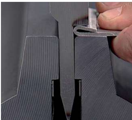
Pre-bend and flattening in the same tool.
